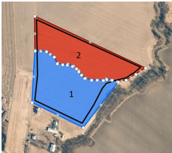
Fig. 5. An example of the prescription map for precision fertilizing of winter wheat with two treatment zones. The zones were fertilized according to the table 1. (Olli Alikärri's field, the plan made with AgriSmart /Suonentieto Oy).
