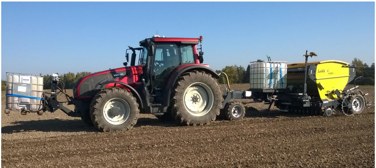
Fig. 3. Industrial IBC chemical plastic containers of 1 m 3 volume used as recycled fertilizer tanks on the machinery work set.
