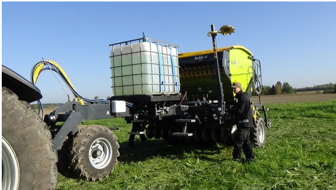
Fig. 7. An industrial IBC container is located on the drawbar of the combined seed driller.
