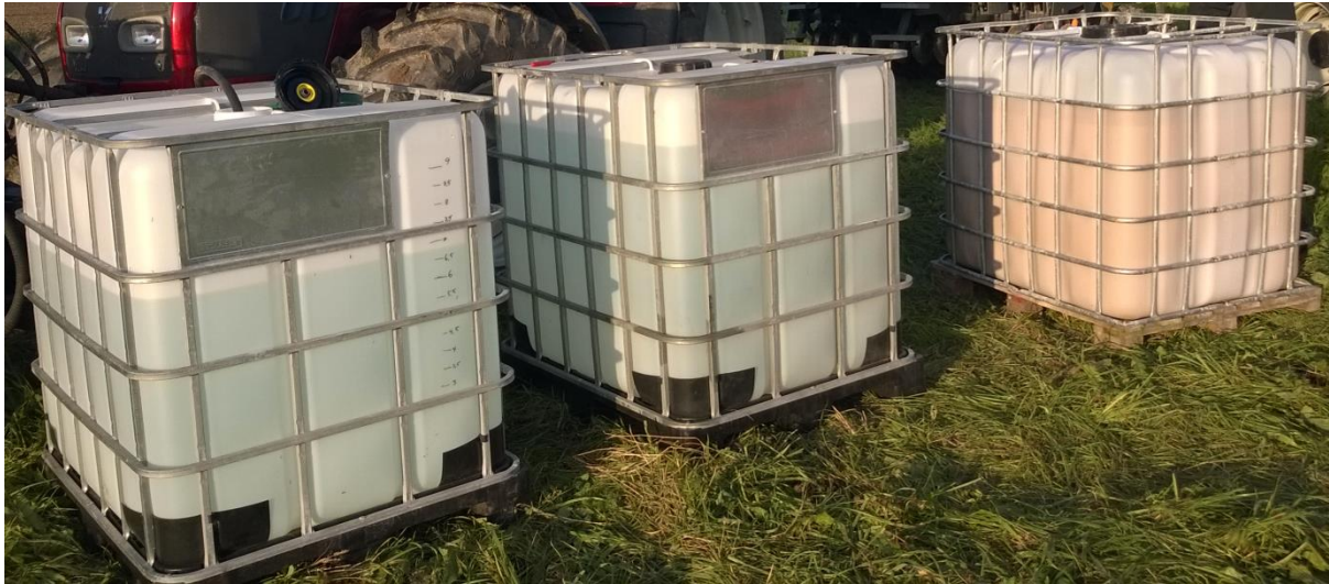
Fig. 2. Industrial IBC chemical plastic containers of 1 m 3 volume used to store recycled fertilizers.
