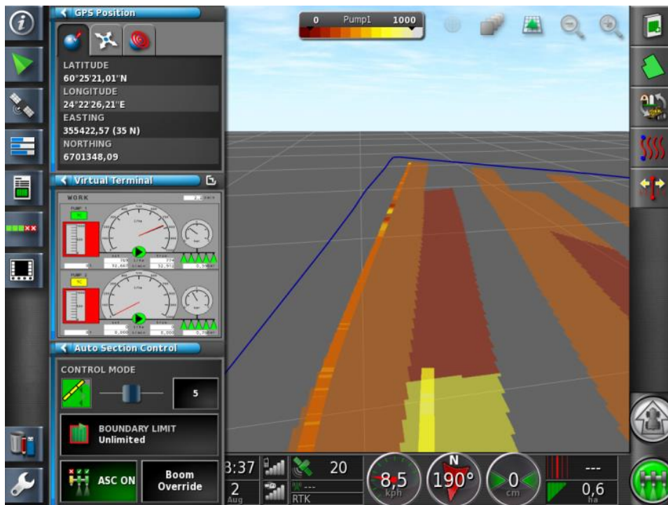
Fig. 8. As an example, ISOBUS compatible Valtra C3000 Task controller as a user interface for the machine combination.
